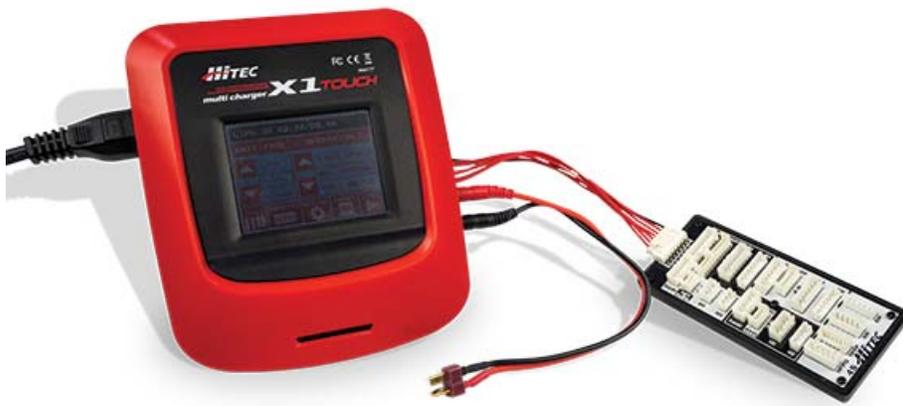
The Hitec X1 Touch AC/DC charger is a 55-watt touch screen charger that is capable of charging one- to six-cell LiPo batteries.
